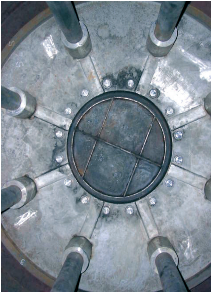
Many coverplate designs are available. This segmented coverplate is designed to accommodate catalyst transfer pipes.
