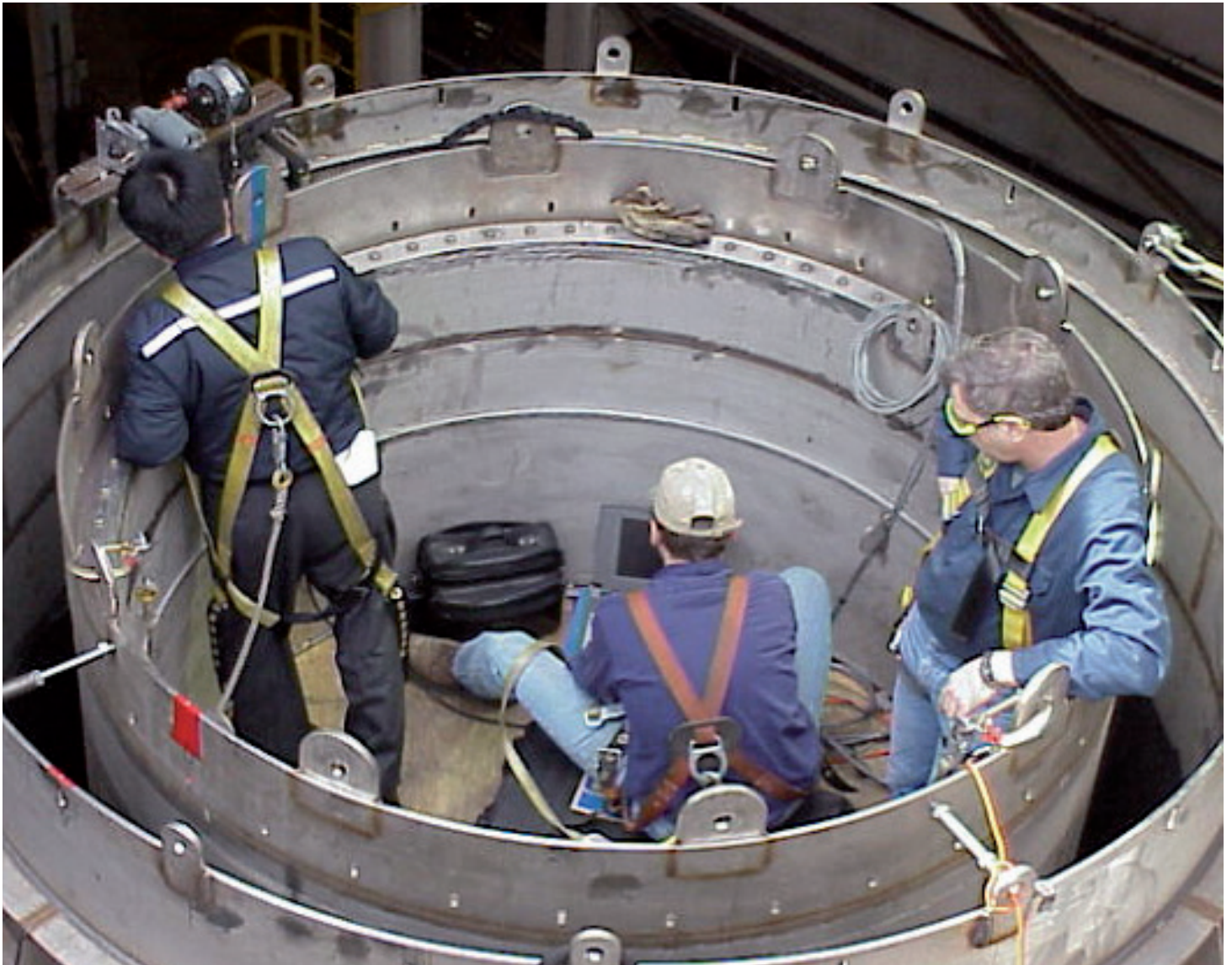
Ultrasonic device allows quick on-site inspection of the annulus between inner and outer screens.
